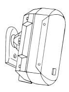
Attaching to a scaffold bar or to a microphone stand by means of the **SM-50** single point mount bracket. For microphone stand use simply remove the microphone clip from the mic stand and locate the threaded end through the hole in the top of the SM-50 bracket. Tighten with the wing nut provided. For use with a scaffold bar, place the bracket over the bar and tighten with the supplied M6 screw until secure.
